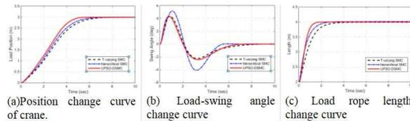
Fig. 1. Results of three sliding mode control anti-swing Positioning Control
